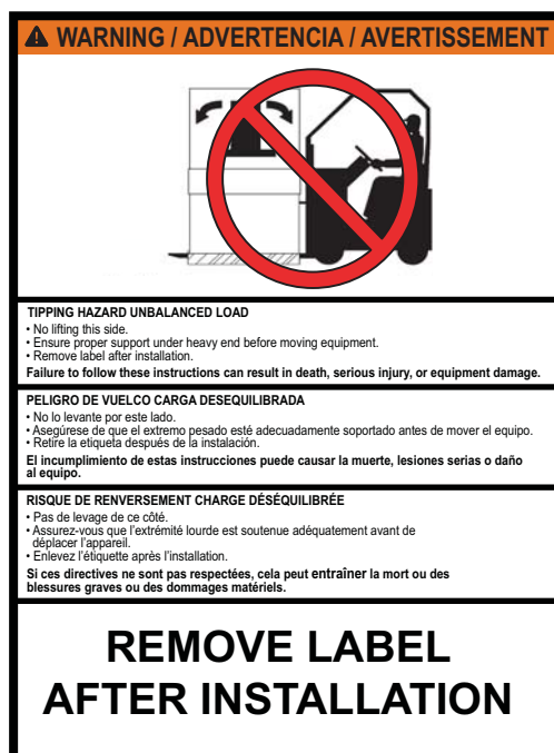
Figure 5 – Front Warning Label, Rainproof Switchboards
