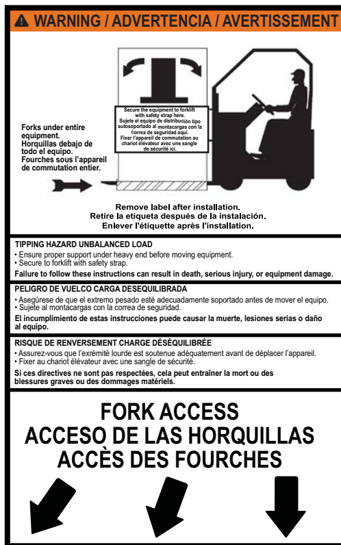
Figure 4 – Rear Warning Label, Rainproof Switchboards
