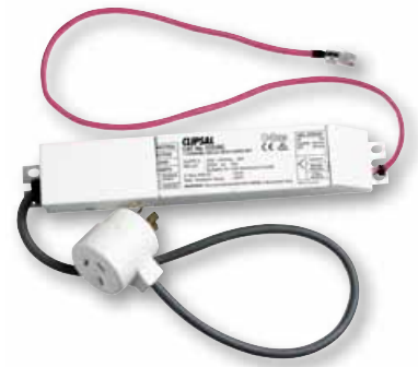
5101RC 1 channel relay 250V ac 10A inductive load, complete with 3 pin mains, flex and plug and C-Bus lead with pre-terminated RJ45 connector
