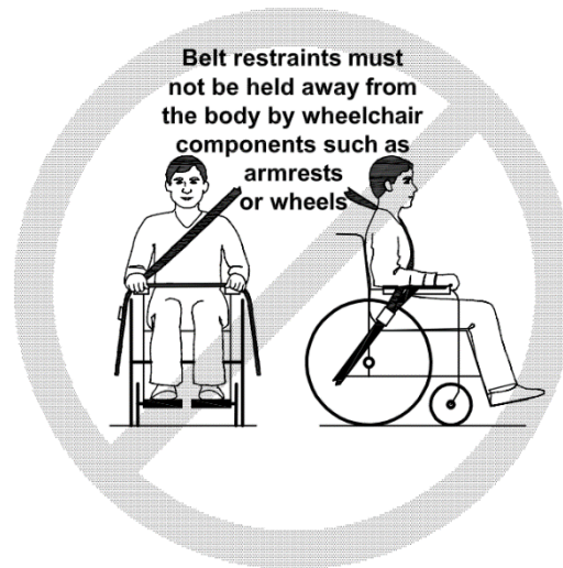
Figure 27 - Improper belt restraint fit
