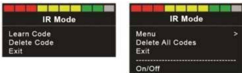
Figure 20 - Deleting individual IR codes (left) and sets of IR codes for an appliance (right)
