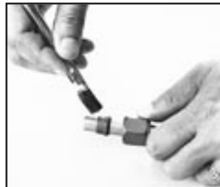
Step 3 – Lubricate ferrule with system fluid or a compatible lubricant.
