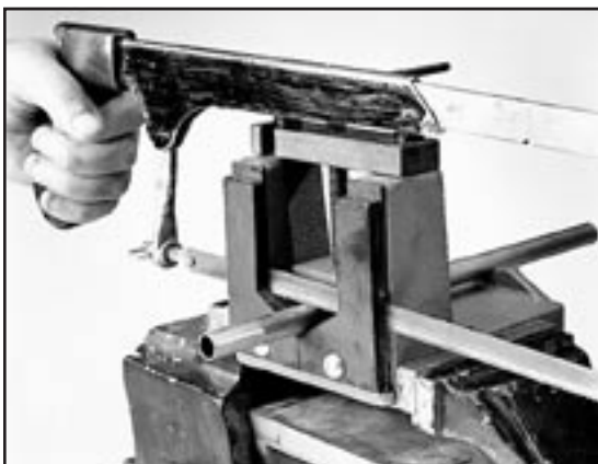
Fig. T11– Parker's Tru-Kut Sawing Vise used with hacksaw
