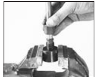
Step 4 – Bottom tube end firmly on internal shoulder of Ferulset Tool (or fitting body).
