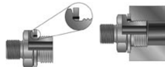
Fig. T5 – Bonded Seal
