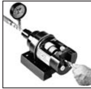
Fig. T26 – Flaring with Hydra-Tool
