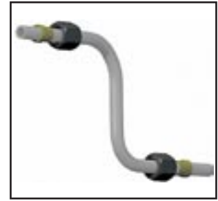
Fig. T27 – Nuts and sleeves assembled before flaring
