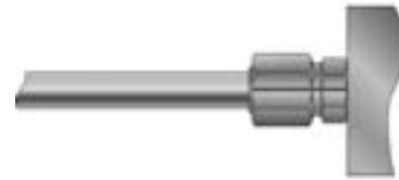
Fig. T31 – Make reference mark on nut and tube body
