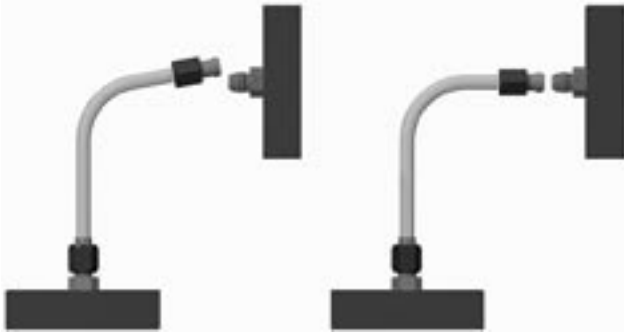
Fig. T30 – Improper bend and short tube
