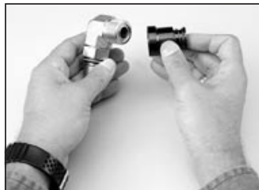
Fig. T24 – O-Ring installation using the CORG assembly tool
