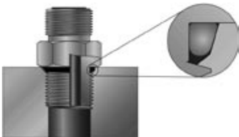
Fig. T1 – SAE / ISO / JIS B2351 Straight Thread Port O-Ring Upon Assembly
