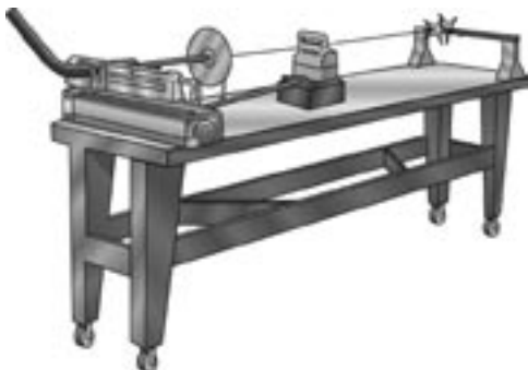
Fig. T55 — Hydraulic bender with portable table for mandrel bending
