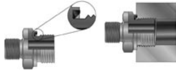
Fig. T2 – EOlastic Seal, Type E
