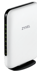
WAP6804 Dual-Band AC2100 Gigabit Wireless Extender
