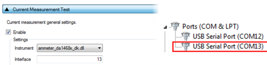
Figure 173: DA1468x DK PRO Current Measurement Settings
