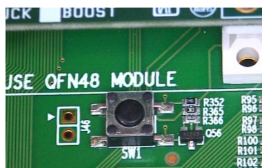
Figure 154: R365 (10 k \Omega ) Added Next to Reset Button
