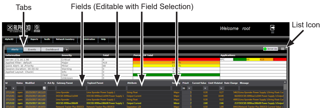
Fig. 4-26, Fault Notifier Page
