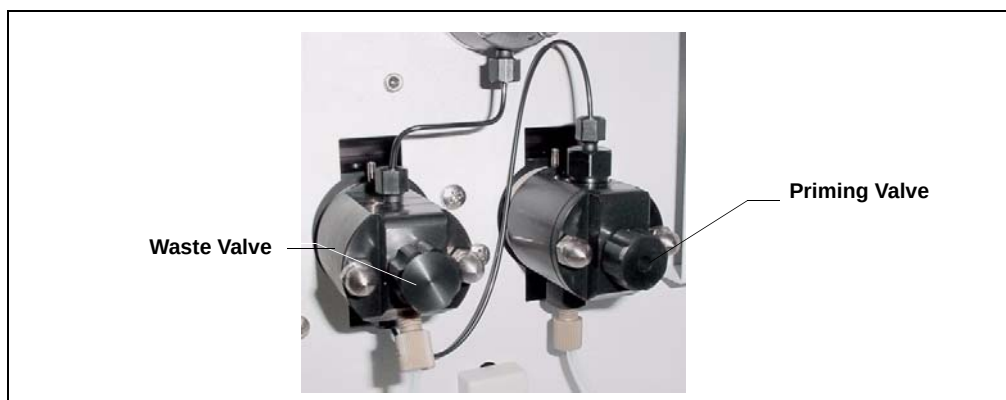
Figure 4-2. Waste and Priming Valves
