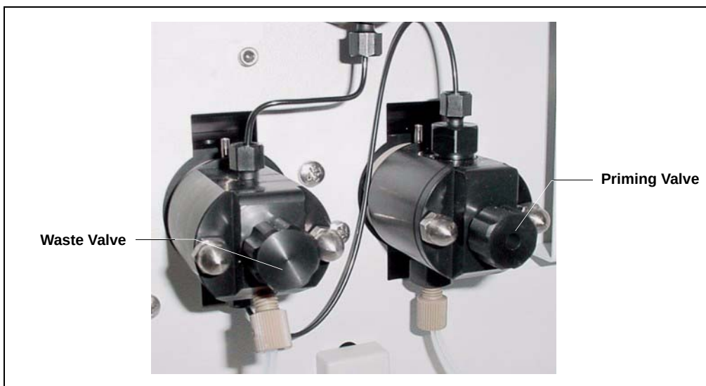
Figure 5-12. Waste and Priming Valves
