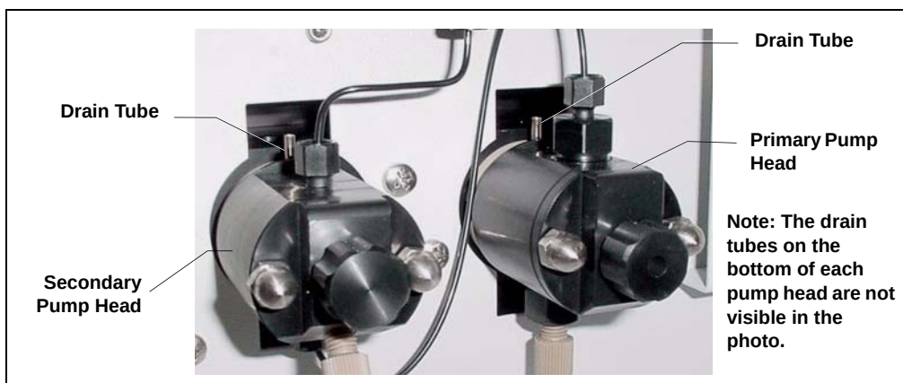
Figure B-48. Primary and Secondary Pump Heads with Drain Tubes
