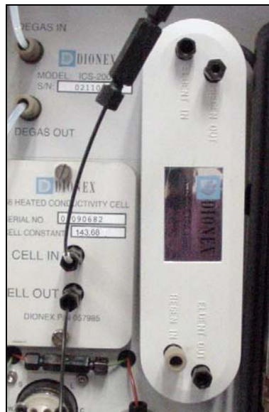
Figure B-21. Suppressor Installed (SRS Shown)
