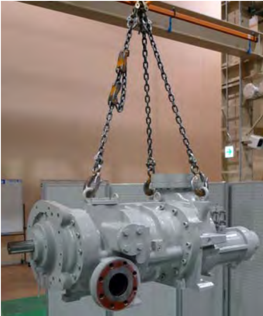
Figure 3-8 Compressor being Lifted
