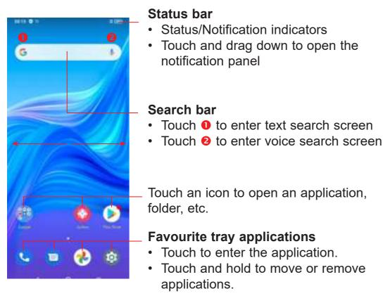
The Home screen is provided in an extended format to allow more space for adding applications, shortcuts etc. Slide the Home screen horizontally left and right to get a complete view.
