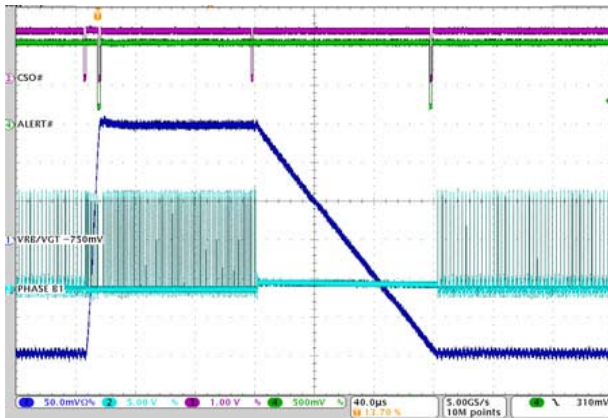
Figure 37. VGT/VR B SetVID_fast, 0.6V to 0.9V, PS0, SetVID_decay, 0.9V to 0.6V, I_O = 2A , R_{LL} = 2.0m\Omega
