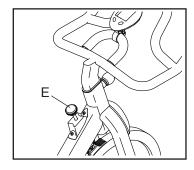
To stop the flywheel, push the resistance knob downward. The flywheel should quickly come to a complete stop.
