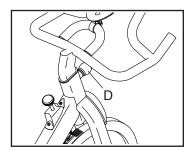
the handlebar, and firmly tighten the adjustment knob. Make sure that the adjustment knob is engaged in an adjustment hole.
