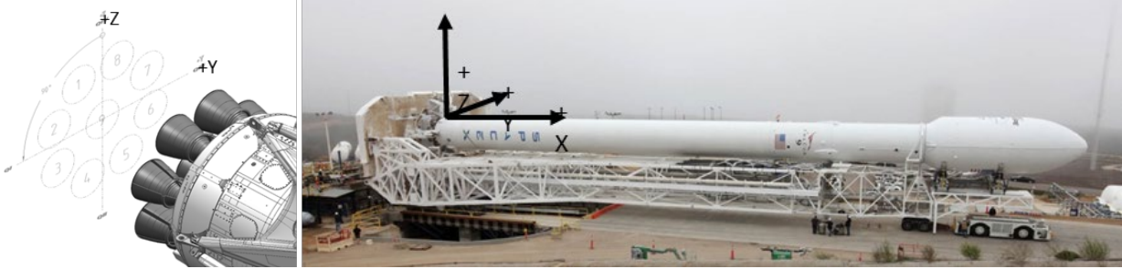
Figure 2-4: Falcon vehicle coordinate frame
