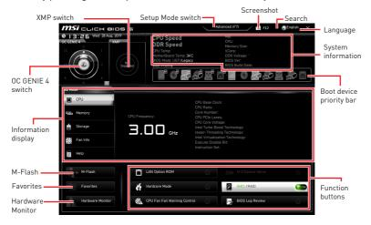
• OC GENIE 4 switch (optional) - click on the center button to switch the OC GENIE 4 be controlled by software (SW) or hardware (HW). The inner circle represents the current stage of hardware OC GENIE 4 and the outer circle stands for software. You can read the abilities of OC GENIE 4 by clicking on the question mark in the rightbottom corner. This function will only be available if the installed processor supports this function
