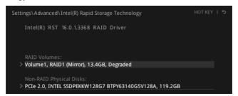
4. Select the Degraded RAID volume from the Intel(R) Rapid Storage Technology screen to enter the RAID VOLUME INFO screen.
