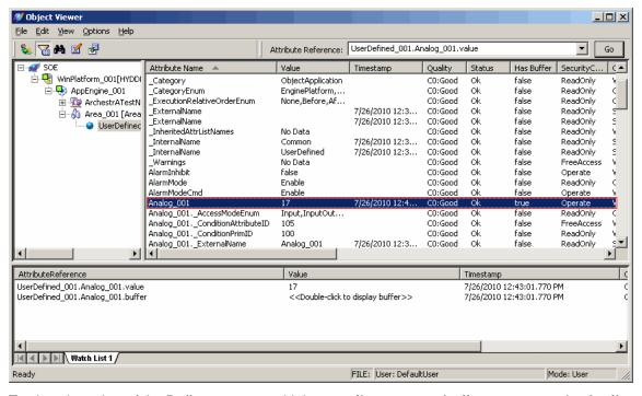
To view the value of the Buffer property, add the **<attributename>.buffer** property to the **Attribute Reference** dialog box. You can also use an alternate syntax, **<attributename>.property(Buffer)**, which should be used for subscribing to attributes on a DI Object.
