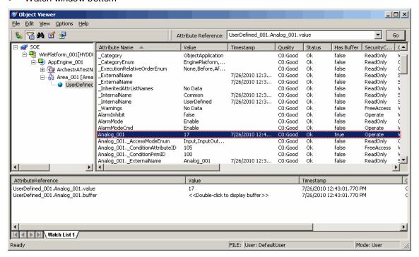
The console tree works like Windows Explorer. Use the plus (+) and minus (-) signs to expand or hide the nested list items shown in the pane. When you select an object in the console tree, its associated attributes and their properties are shown in the details pane.
