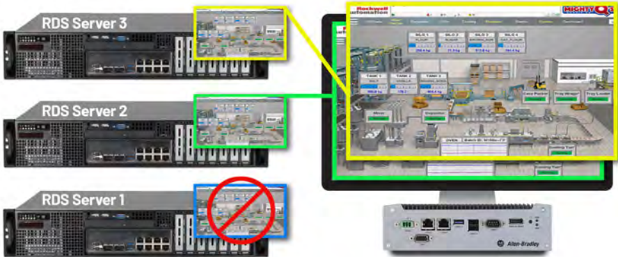
Figure 174 - Terminal with Instant Failover and Backup Sessions
