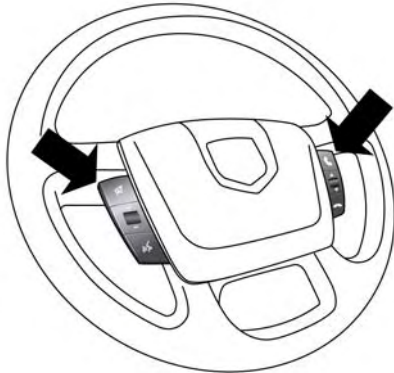
Remote Sound System Controls
