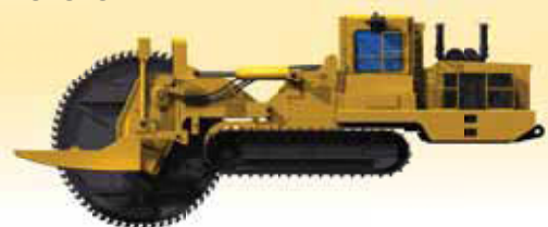
Large Wheel Trencher
