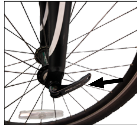
Left: Location of quick release lever on front wheel. Below: Locations of quick release levers on steering columns.
