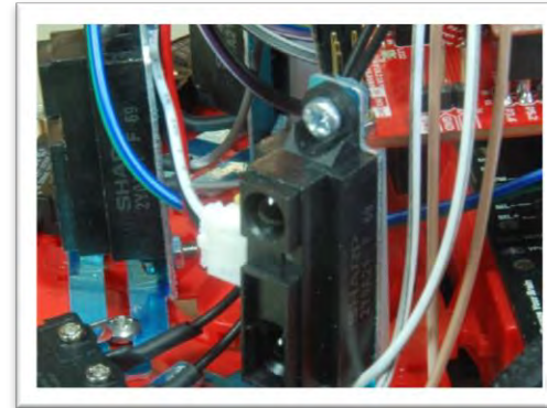
Figure 1. Three IR distance sensors positioned at the front of the robot.
