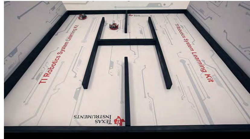
Figure 9. The track is wide enough that the IR distance sensors are monotonic.
