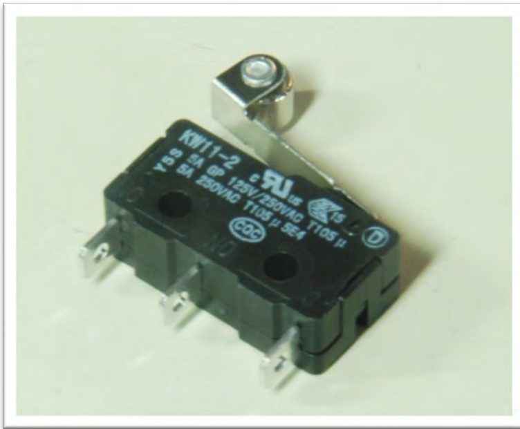
Figure 2. Momentary contact switches allow for collision detection.
