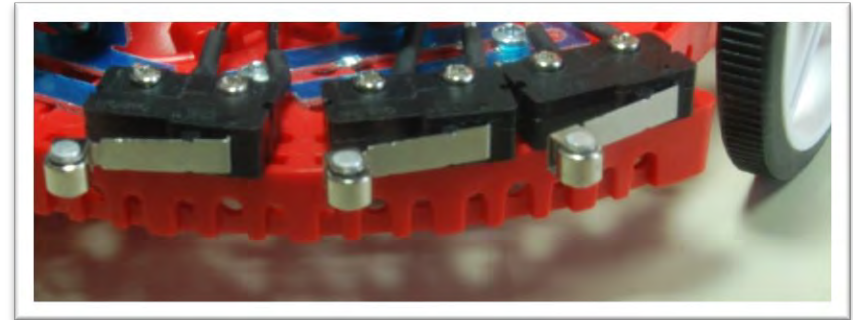
Figure 1. Bump sensors positioned at the front of the robot.
