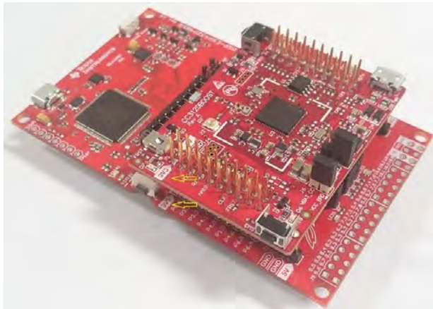
Figure 3. Wi-Fi BoosterPack positioned on top of MSP432 with markers aligned.
