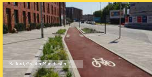
Figure 21. Example of a SUDS segregated cycle track
