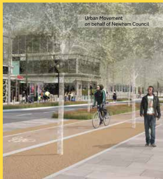
Figure 24. Example of a footpath level cycle track
