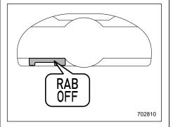
After the brake pedal is depressed, the RAB OFF indicator will illuminate and the system will temporarily stop operating. The RAB OFF indicator will turn off when the select lever is shifted to a position other than the "R" position.
