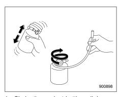
1. Shake the sealant bottle well. Loosen the hose.
