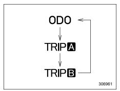
To reset the trip meter, select either the A trip or B trip meter, then press and hold the TRIP RESET switch.
