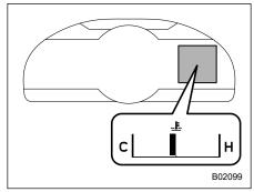
If the radiator cooling fan does not operate even when the engine coolant temperature gauge exceeds the normal operating range, the cooling fan circuit may be defective. Refer to "Engine Coolant Temperature Gauge" P129.
