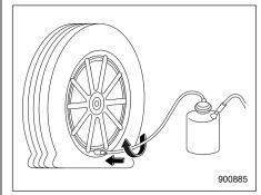
Connect the hose from the bottle to the tire valve stem tightly.
