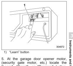
"Learn", "Smart", or "Program" button. This can usually be found where the hanging antenna wire is attached to the motor-head unit (see the device's manual to identify this button). The name and color of the button may vary by manufacturer.
