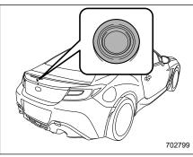
A rear view camera is attached to the trunk lid. When the ignition switch is in the "ON" position and the shift lever (MT models) or select lever (AT models) is set ω to "R", the rear view camera automatically displays the rear view image behind the vehicle on the center information display.
