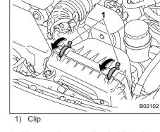
1. Unsnap the two clips holding the air cleaner case (rear).
