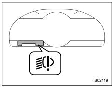
The LED headlight warning light illuminates if the LED headlights malfunction. Have your vehicle inspected at SUBARU dealer as soon as possible.
