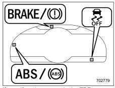
If a malfunction occurs in the EBD system. the system stops working and the brake system warning light and ABS warning light illuminate simultaneously.
