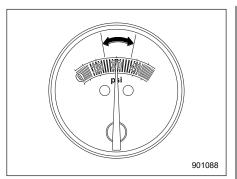
6. Turn the air compressor power switch off when the air pressure reaches the green zone of the air gauge.
