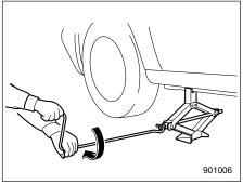
9. Insert the jack handle into the jackscrew, and turn the handle until the tire clears the ground. Do not raise the vehicle higher than necessary.
