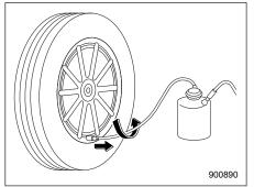
Remove the hose after filling the tire with air and fasten the valve cap.
