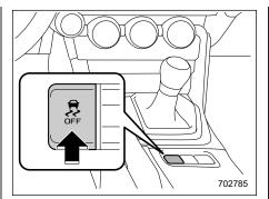
Press the Vehicle Stability Control (VSC) OFF switch to deactivate the TRAC system. Creating adequate driving wheel slip by deactivating the TRAC system may help to recover from the loss of traction. Use the Vehicle Stability Control (VSC) OFF switch as necessary.
