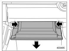
(3) Push both sides of the glove box inward to unlock the stoppers and then pull down the glove box as far as it will go.
