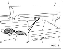
4. Connect the power plug of the air compressor into the accessory power
