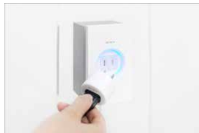
"Authentication outlet," which makes possible the management of electricity on a per-user or per-device basis
