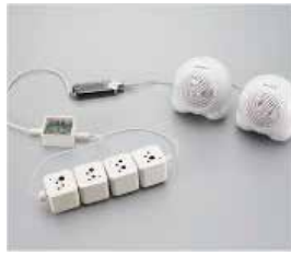
Powering a Walkman digital music player using a prototype bio battery that generates power from a glucose solution (February 2009)
