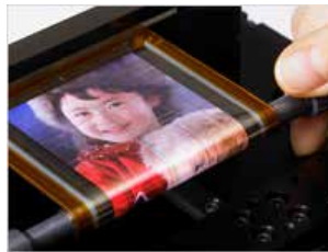
An organic TFT-driven EL display prototype that can be rolled up (May 2010)
