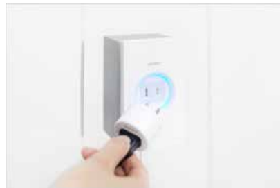
Prototype of Sony's new Authentication Outlet, which enables users to identify electric power fees on a per-device basis
