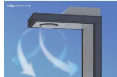
Air curtain creating dome-shaped cooling space
