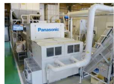
Near-infrared sorting machine that can sort three types of resin simultaneously
