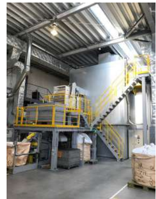
Compact crushing and sorting system for heat exchanger of air conditioner in PETECK
