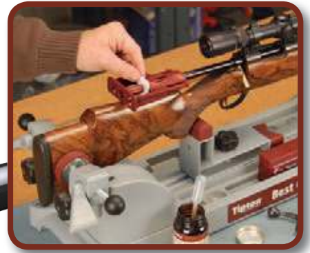
1. With the sliding rear guide pulled out, center the patch with access hole
