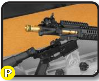
Bore Guide centers cleaning rod in chamber
