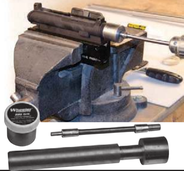
Use the Pic Rail of an AR Upper or other device to mount into your bench vise
