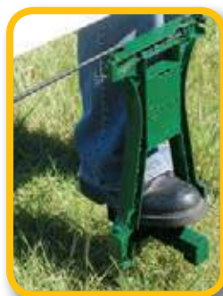
Use your foot to drive the spike into the ground.
