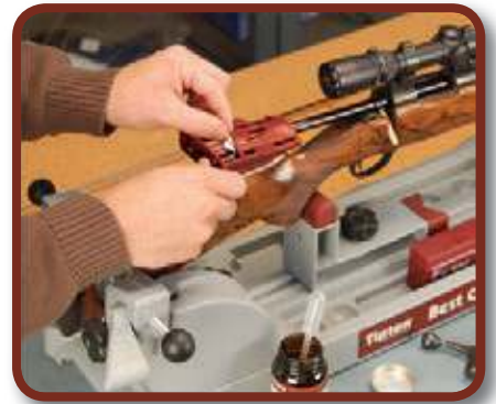
2. Push the sliding rear guide forward, securing the patch
