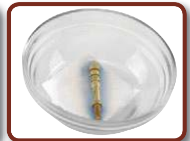
It's apparent that brass jags ultimately contribute to false blueing on your cleaning patches.
