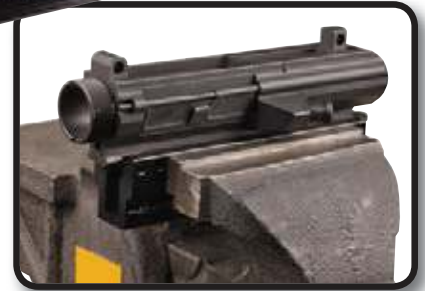
Use the Pic Rail of an AR Upper or other device to mount into your bench vise
