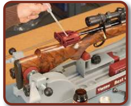
3. Use the built-in solvent port to apply solvent to the cleaning patch
