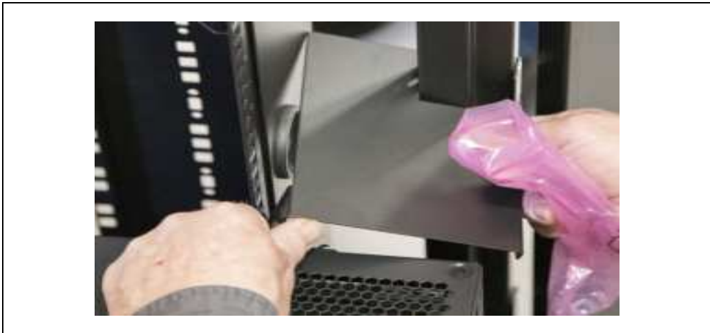
Figure 4.2 Attach Air Baffles—800 mm (31.5 in.) Rack
