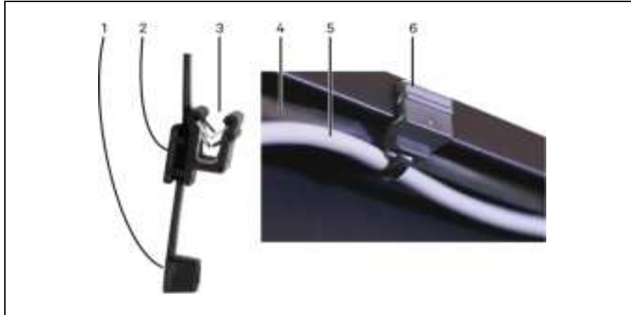
Figure 4.7 Secure the Local Display and Fan Cables
