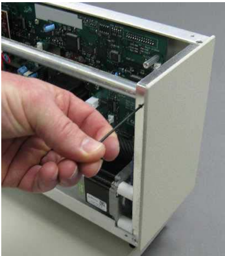
Figure 1-29 Loosening of guide shaft set screws (ASX-260).
