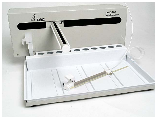
Figure 1-7 Z-drive removed from arm assembly (ASX-520).
