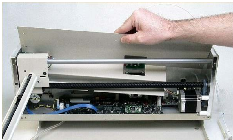
Figure 1-18 Removal of inner shield (ASX-520).
