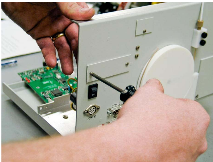
Figure 1-36 Removal of access plate (ASX-260).
