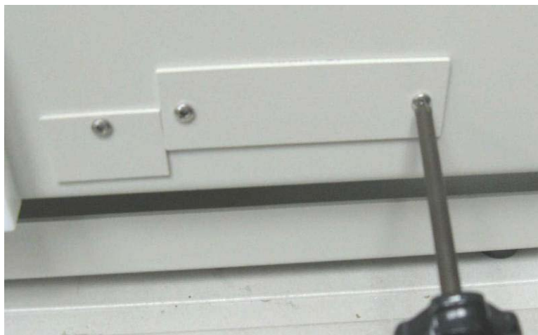
Figure 1-20 Removal of ASX-520 auxiliary connector cover plate.
