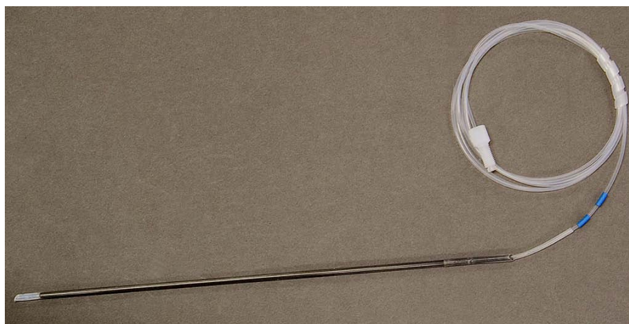
Figure 1-48 Double Blue Bands Identify the 1.0mm I.D. Sample Probe (carbon fiber probe shown is standard equipment)
