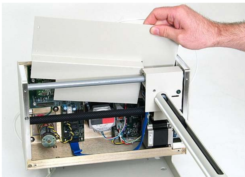
Figure 1-19 Removal of inner shield (ASX-260).
