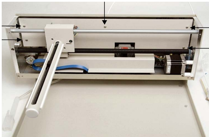
Figure 1-16 View of inner shield inside the ASX-520 Autosampler.
