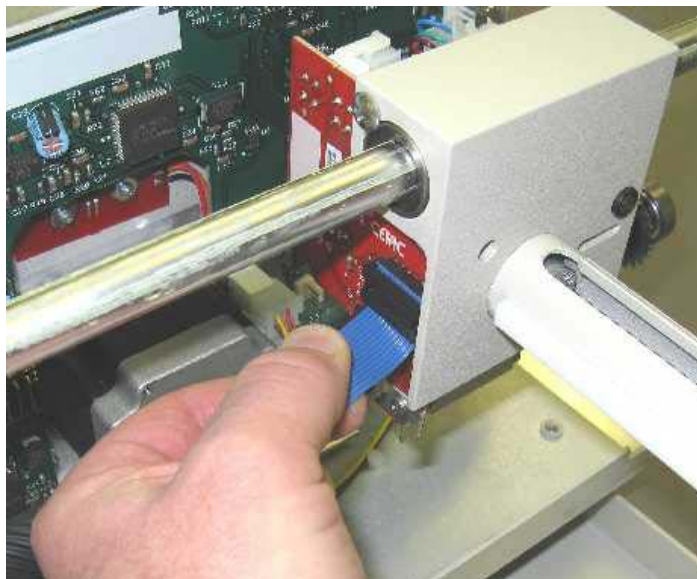
Figure 1-28 Removal of blue ribbon cable from carriage (ASX-260).
