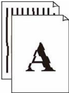
Lines Are Misaligned/Distorted
