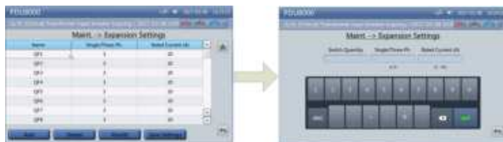
Figure 8-24 Adding an MCB
