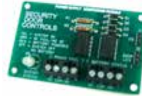
PSM Power Supply Remote Monitoring Module
