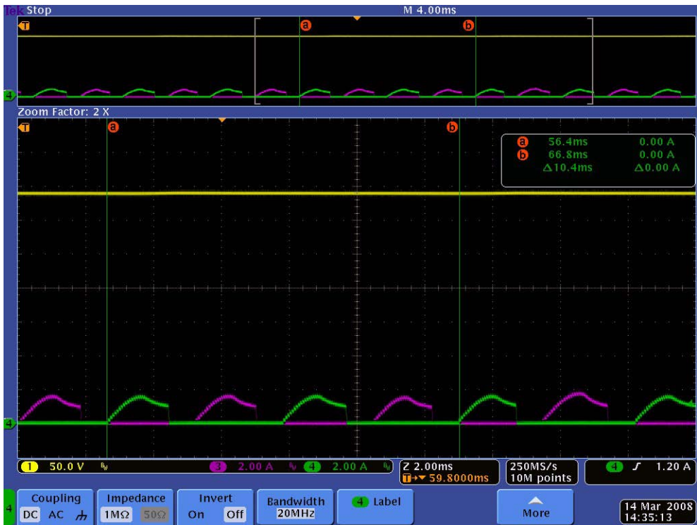
Figure 5-6. SR motor operation at low speed (5700 RPM)
