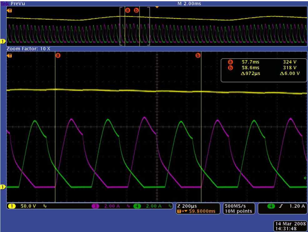
Figure 5-7. SR motor operation at maximal speed (61 000 RPM)
