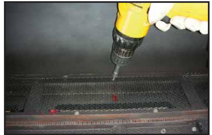
Figure 5. Removing Screws from Basepan.
