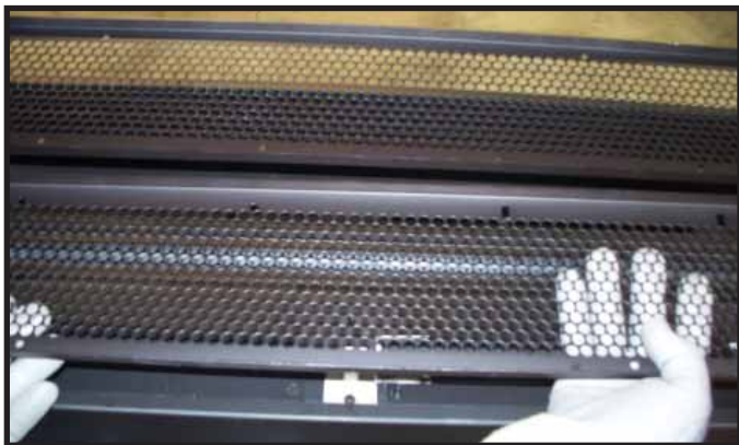
Figure 8.10 Lifting Base Pan Up and Out.
