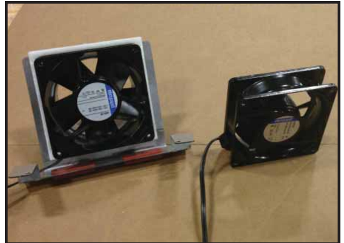
Figure 8.21. Proper Blower Mounting.
