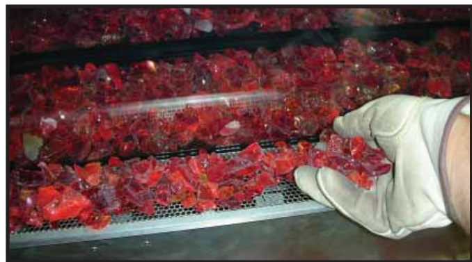
Figure 8. Placing Rock Media in Front Tray.
