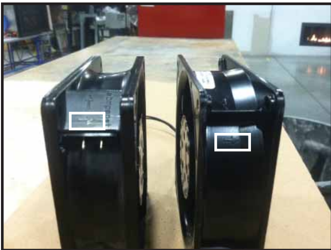
Figure 8.20. Arrow Indicates Direction of Air Flow
