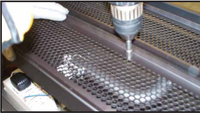
Figure 8.9 Removing Screws from Base Pan
