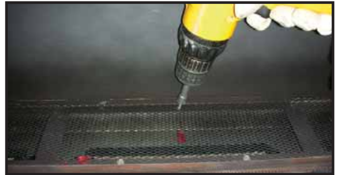
Figure 9. Removing Screws from Basepan.
