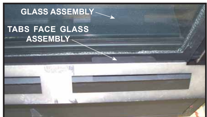
Figure 12. Positioning Porcelain Access Panel.
