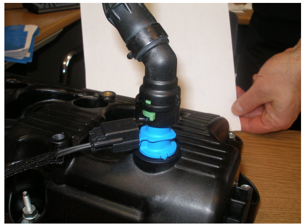
Assembled PCV system
