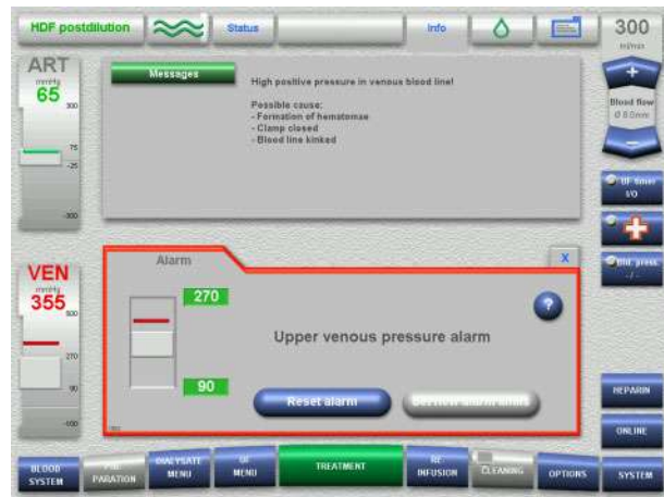
Alarm message (Info window at the top opened)
