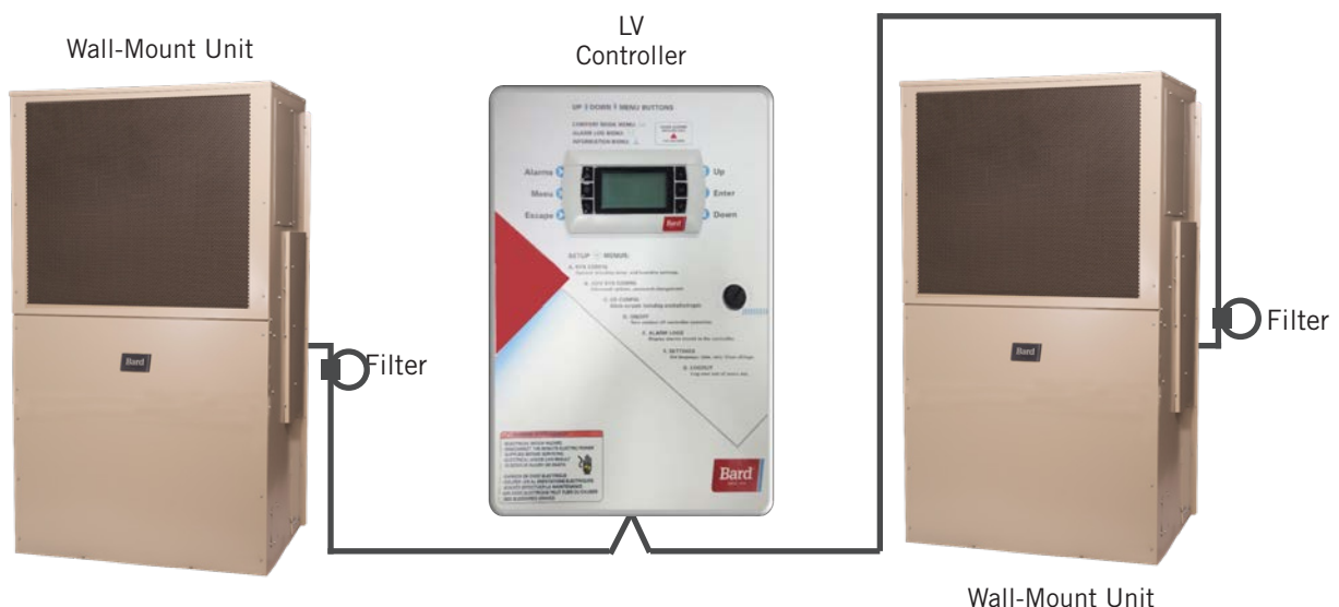
FIGURE 27 Communication Wiring (Alternate Method)
