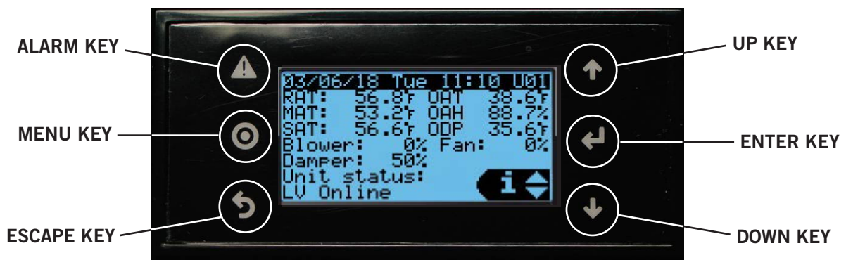
FIGURE 36 TEC-EYE (Bard P/N 8301-059) Display and Interface (Status Screen Shown)
