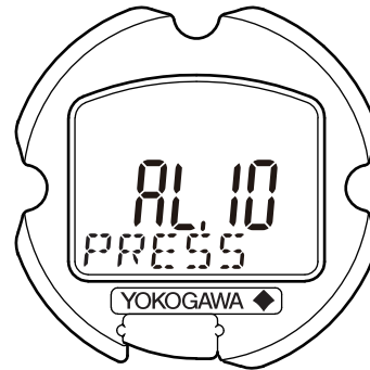
Self-diagnostic error on integral indicator (Faulty transmitter)
