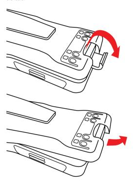
To re-fit the battery pack, slide the top of the battery pack in towards the radio then press the base of the battery pack downwards against the battery contacts. Rotate the battery lever upwards and press into place so that it clicks firmly.
