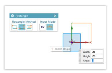
6. Finish the sketch. Name the sketch 'Robot base'. Adjust the view by selecting the View menu, then Fit to Window. You can use your mouse roller to zoom in or out, or alternatively, select view options by right clicking on your work area.
