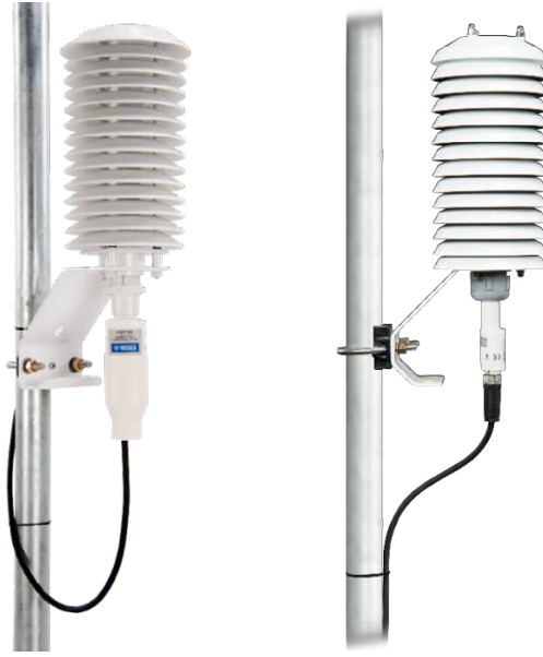
FIGURE 7-5. HMP155A and 41005-5 14-plate radiation shield (left) and RAD14 (right) on a tripod mast
