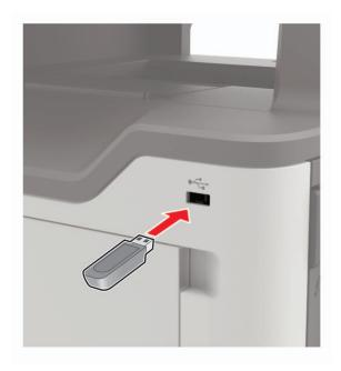
**3** Touch **Scan to USB** and adjust the settings if necessary.
