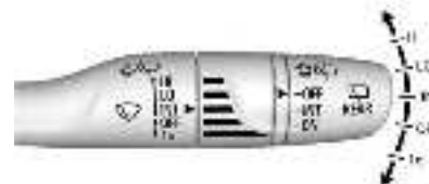
Windshield Wiper with Intermittent Wipes (INT Shown)
