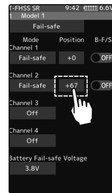
Fail-Safe position setting While holding the wheel or trigger, tap the Fail-Safe position button.
