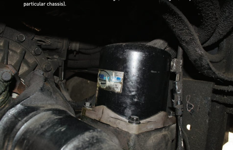
Above: The air dryer on this Tiffin Phaeton is mounted on the driver's side frame rail just behind the rear axle. Shown is the top housing of a Haldex air dryer. Below: Under the black canister is the desiccant air filter cartridge, which should be changed (every 36 months on this particular chassis).
