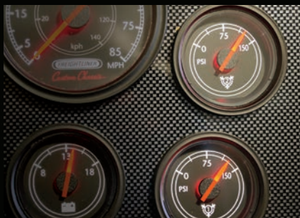
Above, left: This is what a typical air gauge set looks like on a motorhome. This Freightliner chassis has two tanks and two pressure gauges labeled 1 and 2. The gauges are displaying the normal operating pressure of 125 psi. Above, right: This is a typical brake cylinder mounted to the caliper on a front wheel disc brake. This motorhome has drums on the rear. With disc brakes, the brake cylinder is mounted directly to the caliper assembly.
