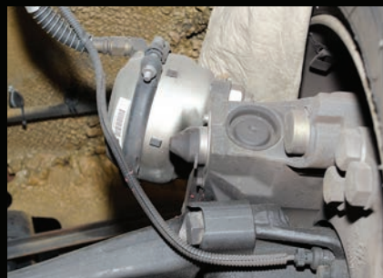
Above, left: This is what a typical air gauge set looks like on a motorhome. This Freightliner chassis has two tanks and two pressure gauges labeled 1 and 2. The gauges are displaying the normal operating pressure of 125 psi. Above, right: This is a typical brake cylinder mounted to the caliper on a front wheel disc brake. This motorhome has drums on the rear. With disc brakes, the brake cylinder is mounted directly to the caliper assembly.
