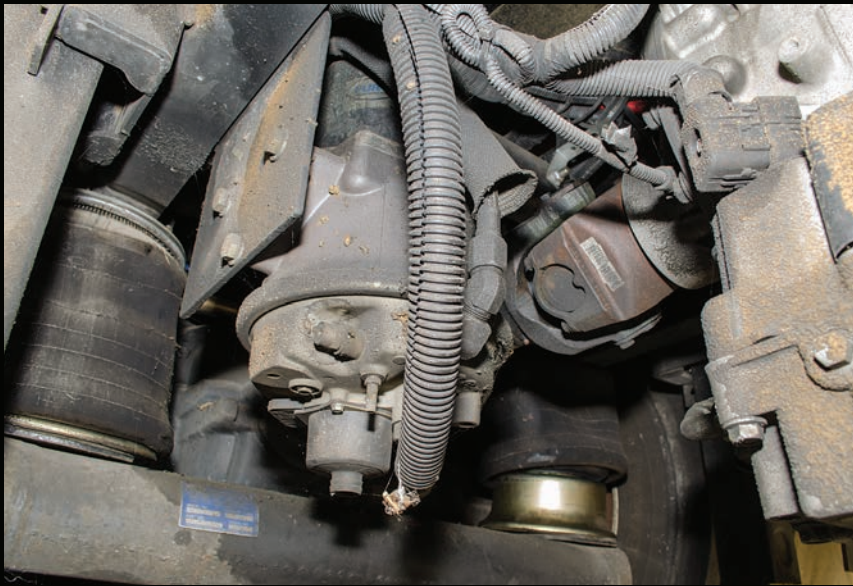
Above: The air dryer on this Tiffin Phaeton is mounted on the driver's side frame rail just behind the rear axle. Shown is the top housing of a Haldex air dryer. Below: Under the black canister is the desiccant air filter cartridge, which should be changed (every 36 months on this particular chassis).
