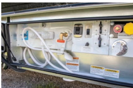
Clockwise, from above, left: The Firefly Integrations multiplex system offers quick access to the Wonder's electronic controls and systems. Space beneath the entry steps allows placement of footwear to help keep the living compartment uncluttered. An exterior shower, plus water, LP-gas, sanitation and winterization systems, are easily accessible behind a compartment door.
