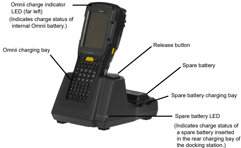
Figure 4-9 Desktop Docking Station - Models ST4002 and ST4003
