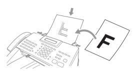
■ The ADF (automatic document feeder) can hold up to 30 Pages, feeding each one individually through the machine. If you "Stagger" the pages, the ADF can hold up to 50 pages. Use standard (17 lb–24 lb) paper when using the ADF. If you're using heavier paper, feed each sheet individually to prevent paper jams.
