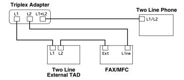
You can keep two-line telephones on other wall outlets as always. There are two ways to add a two-line telephone to the machine's wall outlet. You can plug the telephone line cord from the two-line telephone into the L1+L2 jack of the triplex adapter. Or, you can plug the two-line telephone into the TEL jack of the two-line TAD.
