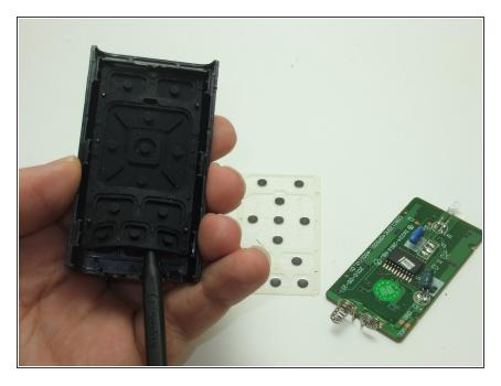
Using either end of the spudger, lift and remove the rubber keypad.
