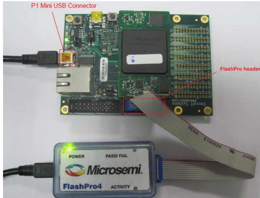
Figure 61 • SmartFusion2 Starter Kit Setup
