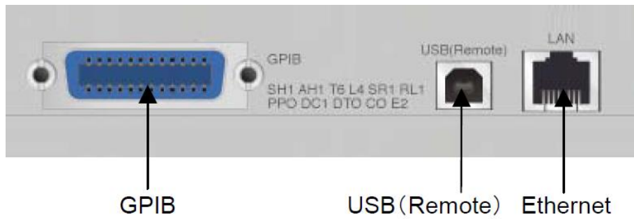
Figure 2 Measuring Instrument Built-in Remote Control Interfaces
