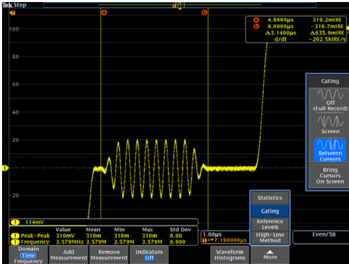
Figure 9. An example of amplitude measurements on an NTSC signal. The peak-to-peak amplitude of the color burst is measured with the oscilloscope's peak-to-peak measurement. The area of the waveform the measurement is being taken on is gated by the cursors.
